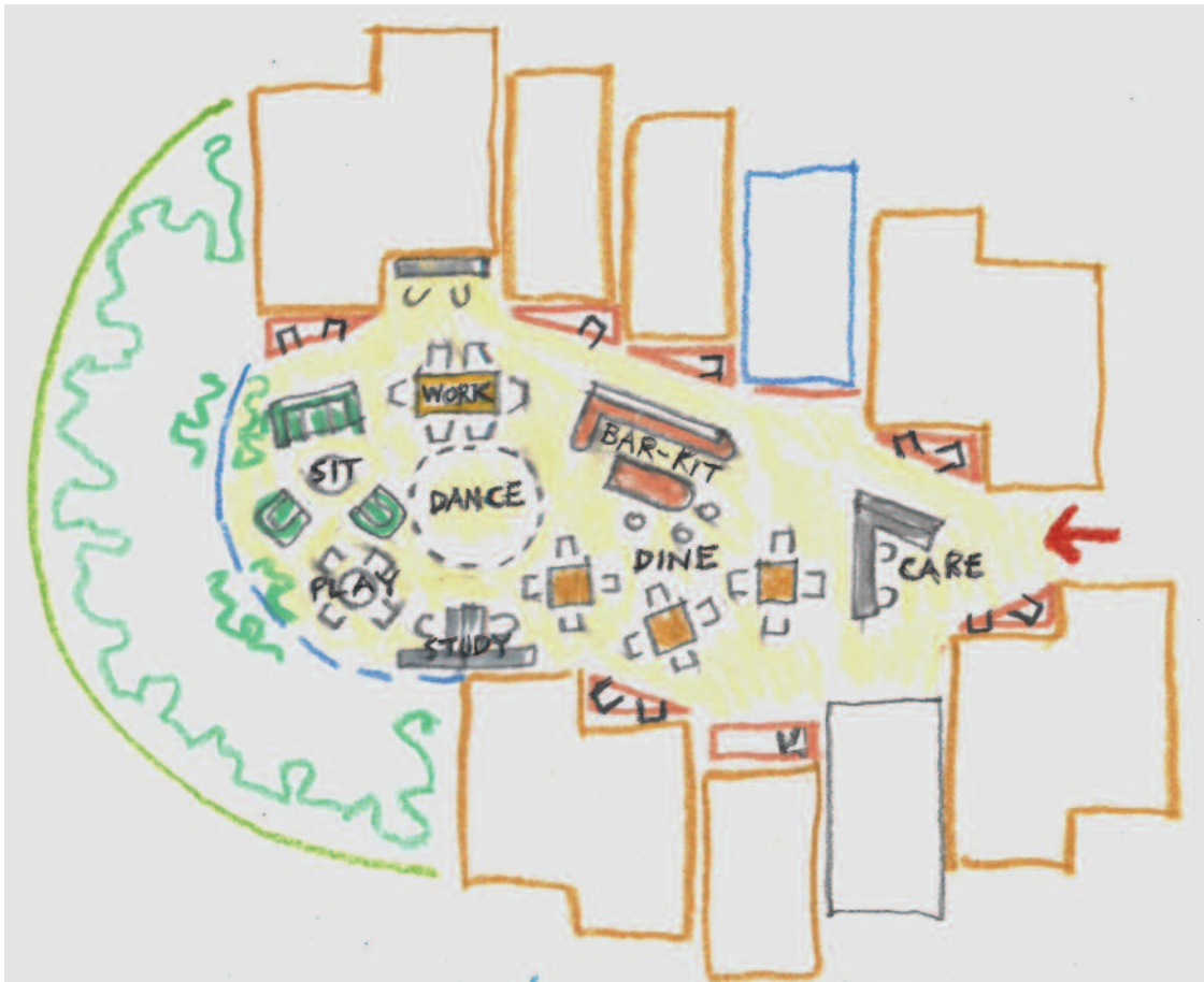
Left: The main activity area must provide space for a social group of 10 to 12 residents with two staff and trained volunteers. Different activities must be clearly identified by means of lighting, colour, decoration, furniture and fittings
